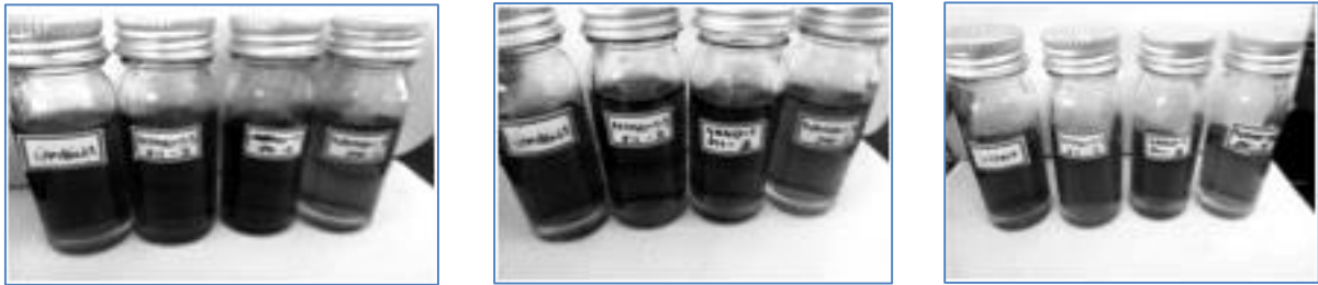
Figure 7 : Treatment of waste water (Sample 3) using Zero Valent Iron Nanoparticle
