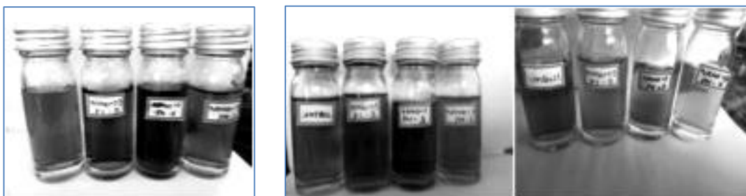
Figure 6: Treatment of waste water (Sample 2) using Zero Valent Iron Nanoparticle
