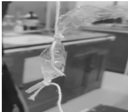
Fig 7 Dialysis Bag with cry Protein SDS PAGE
